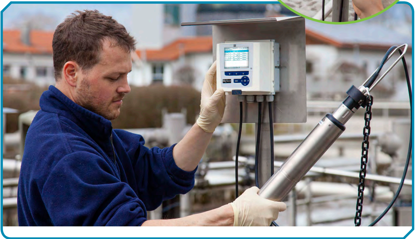
282/284 Terminal Controller with 3 sensors
