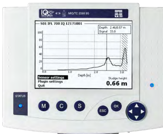
IQSN 2020 3G Controller showing IFL measurements
